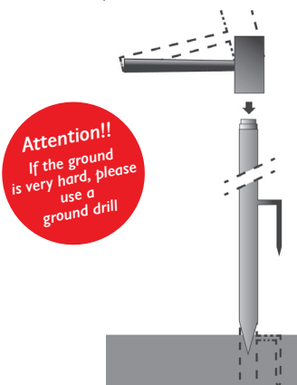
Figure 2: Hammer the base pipe into the ground (with Anti-rotation anchor)
